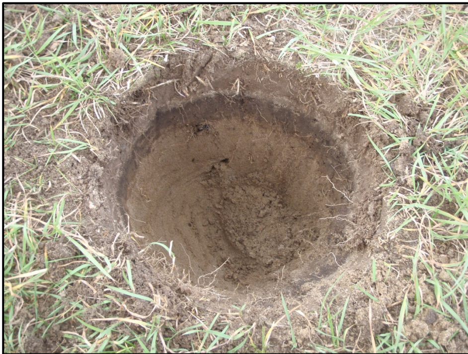
Image 35: Deep Test Pit on Inside Portion of Track, Showing Top Layer of Disturbed Gravel Fill
