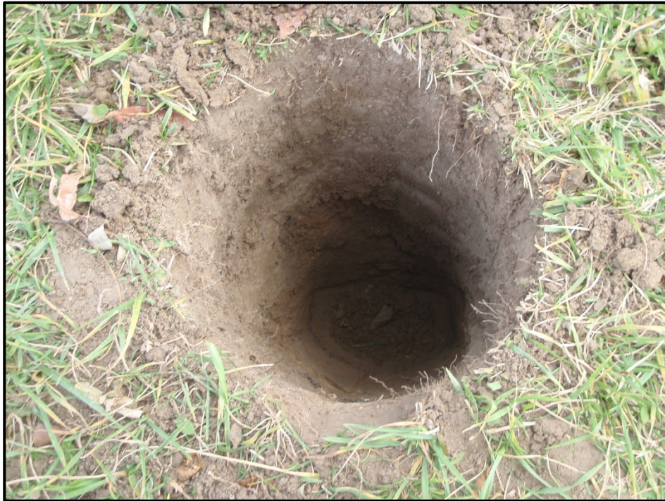
Image 36: Deep Test Pit Showing Beach Sand with Pockets of Loamy Sand
