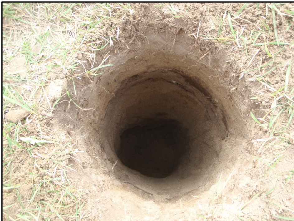
Image 37: Typical Test Pit on Grassed Easement at North End of Connaught Park
