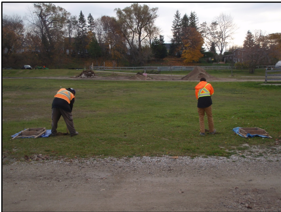
Image 33: Typical Test Pit in Grassed Area of Park, with Orange Sandy Clay
