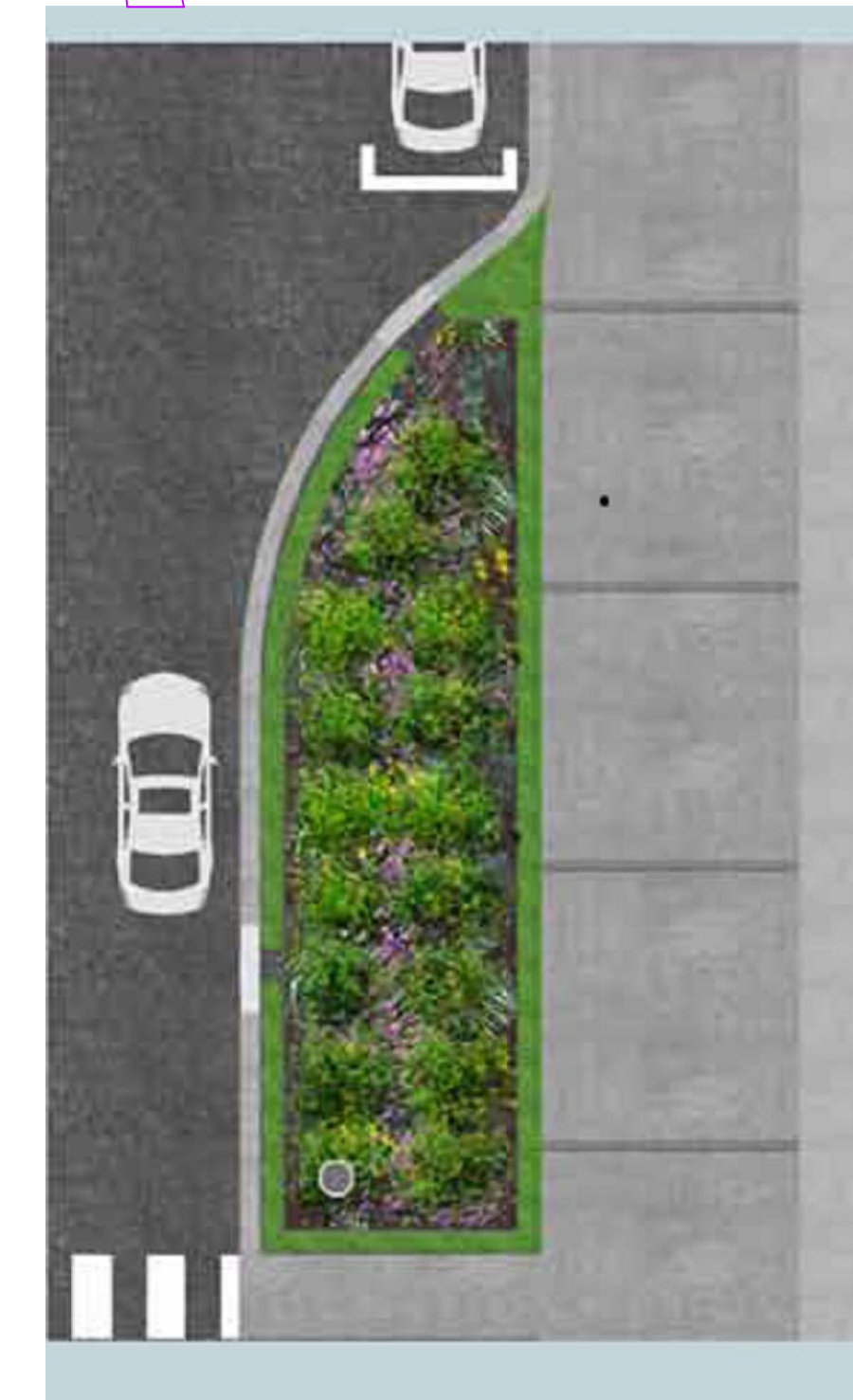
BIORETENTION CURB EXTENSION
