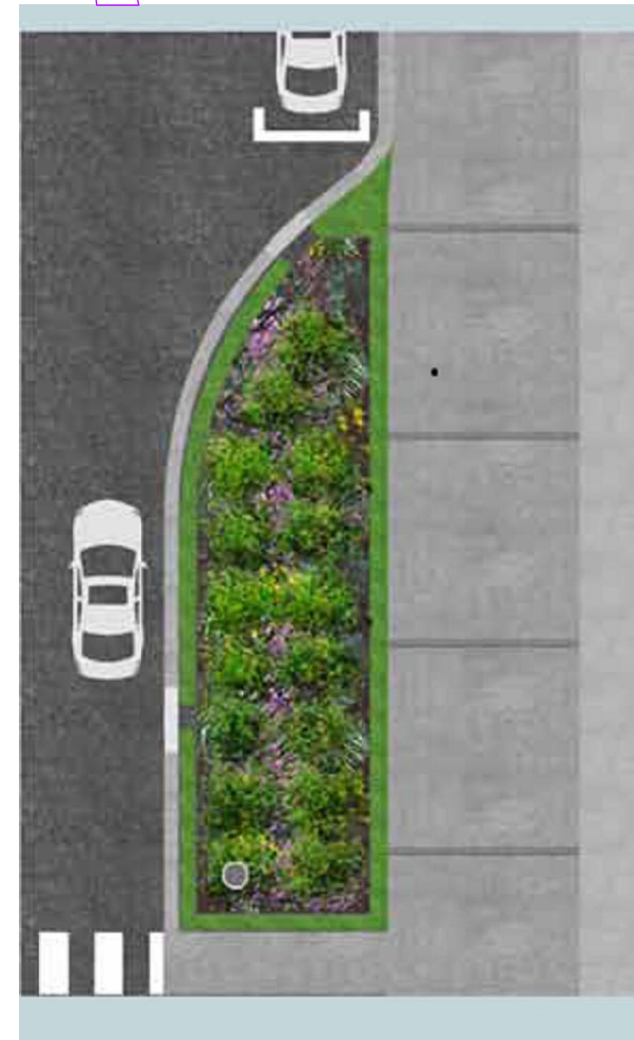
BIORETENTION CURB EXTENSION
